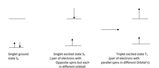
The excited species can return to the ground state by losing all of its excess energy by any one of the paths shown in Jablonski diagram.
